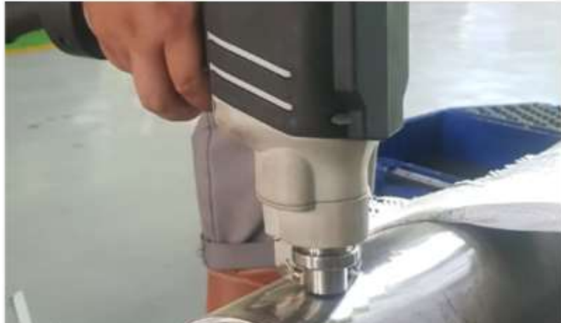
Incoming Material BEFORE PROCESS with PMI XRF Metode
