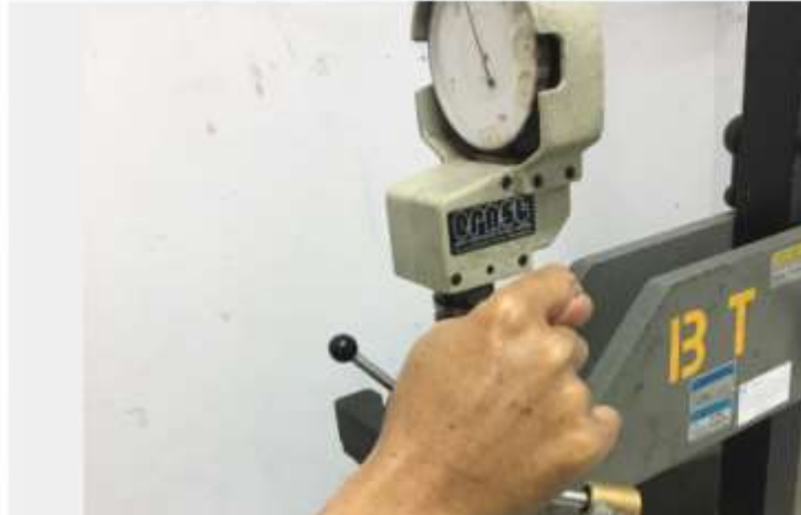
INSPECTION HARDNESS BEFORE NEXT PROCESS MACHINING
